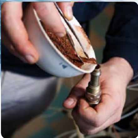
Finely ground adsorption media is placed in a high pressure column in preparation for small scale column testing of its ability to remove arsenic from drinking water.
